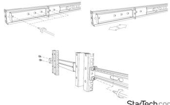
3. Tighten the screws that were loosened in Step 1:
